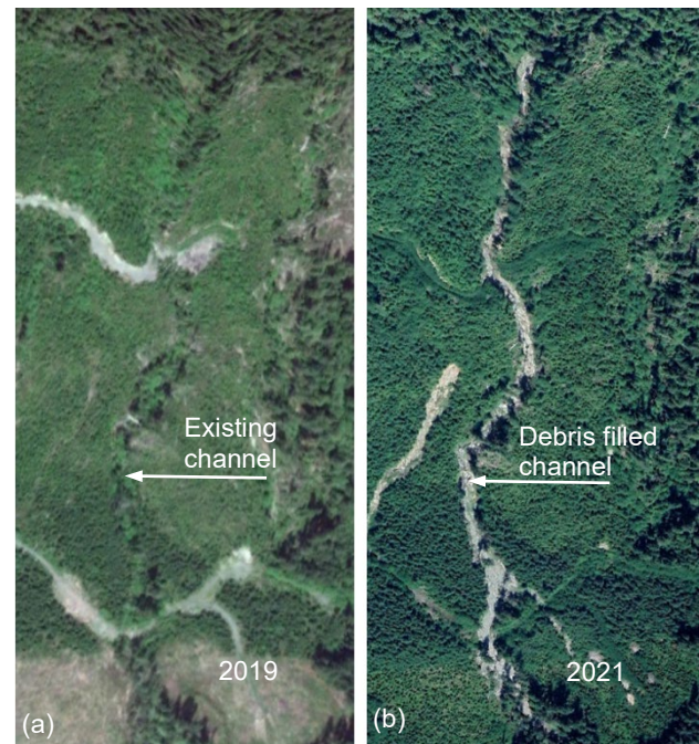
Figure 3: Satellite image along the flow path of C2: (a) image in 2019; (b) image in 2021.
